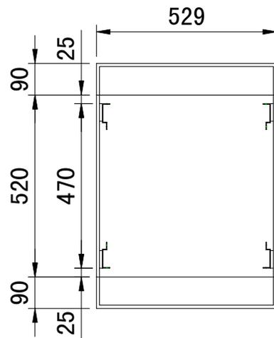
9mm plywood, front and rear with rack rail with square holes,
